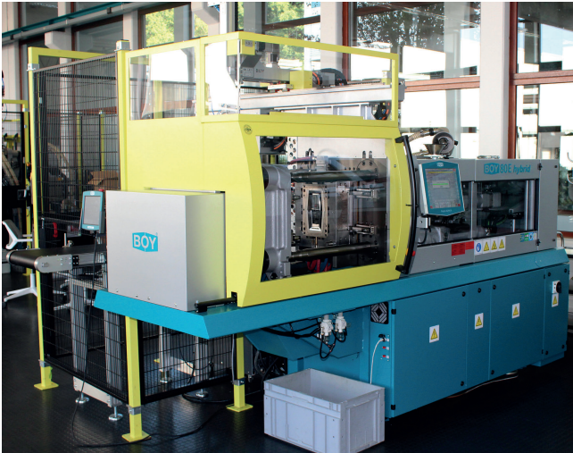
Fig. 2. A Boy 80 E hybrid machine produces beautiful designer plates from so-called Ocean Plastic collected by Tide Ocean SA © Dr. Boy
